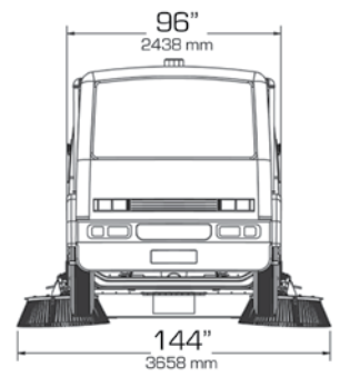
*TYPICAL MEASUREMENTS SHOWN, EXACT DIMENSIONS DEPENDING ON OPTIONS AND TRUCK MANUFACTURER
